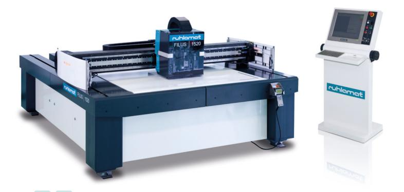
Filus 1520 is a wire embedding system for 2D applications and product sizes up to 1500mm x 2000mm (others on request). By integrating different tools and technologies, the production of complete electrical units is possible. A typical application for the Filus1520 in the automotive sector is the wiring of antennas for manufacturing of car windscreens.
