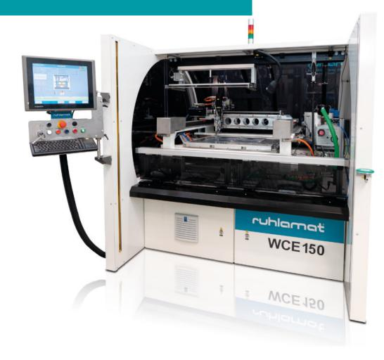
WCE150 is designed for wire embedding for 2D applications. Based on a single-station concept with manual load and unload, it is a convenient solution for small production volumes with a working area of approx. 600mm x 600mm.
