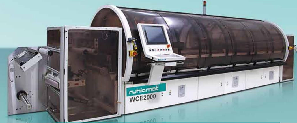
Flexible platform for antenna embedding and RFID inlay production.
