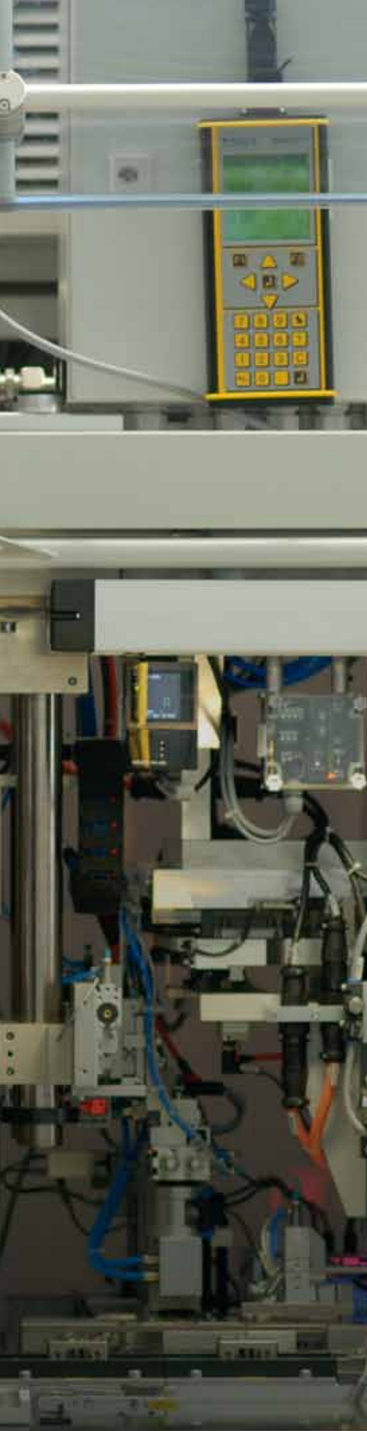
Linear transfer systems, e.g. ruhlamat Compact Carrier System (CCS) 140, allowing workpiece carrier change < 1 sec
