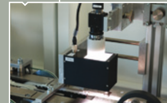
Optical inspection – symbol Optical inspection of the ICCID to check if the data correspond to pre-defined characteristics. Automatic separation of reject cards.
