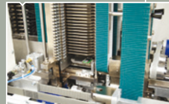
Multiple personalization unit 80 contact heads in one station to contact and personalize 80 modules simultaneously. The MPU handles the cards in a patented flow (Patent Application No. DE102007046141.2)
